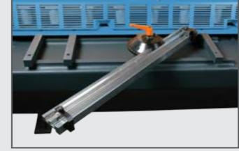
Protractor for Angle Shearing.
