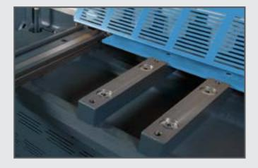
Ball transfers mounted in the iron table blocks, for easy feed-in of the sheets.
